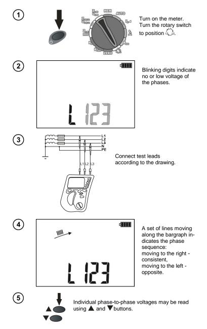
After a few seconds or after pressing **ESC** button, the meter returns to displaying the phase sequence.
