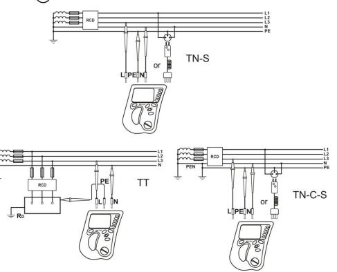
Remaining issues connected with the measurements are the same as those described for measurements of the L-PE circuit.
